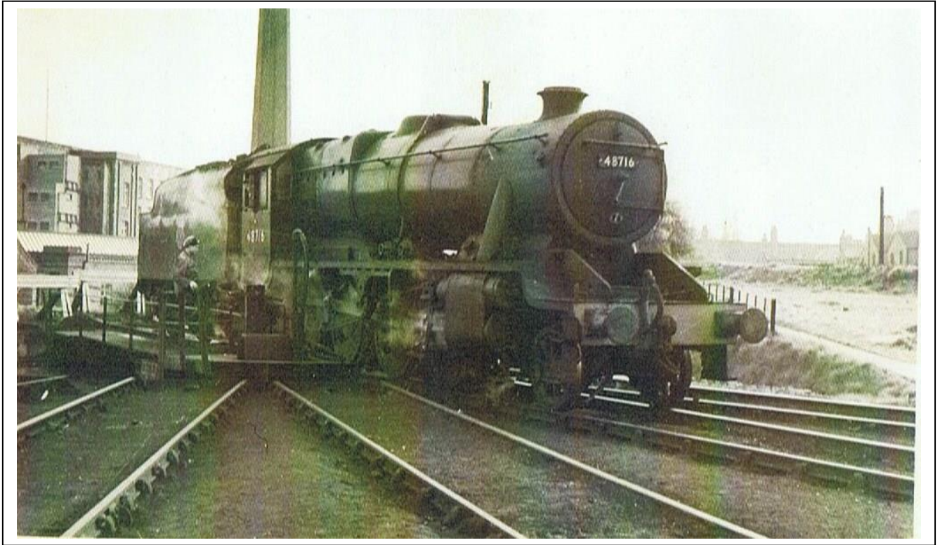
L.M.S. Class 8F 2-8-0 Nr. 48716 drawing forward from the turntable at the rear of Nuneaton shed. In the background Fielding Johnson's mill can be seen. At one time a siding led down to the mill known as the "cotton hole siding". It was used to take coal down for the steam boilers whose enormous chimney can be seen behind the engine. Its name "cotton hole" arose from the fact that Fielding Johnson's mill was built as a cotton mill; it later went over to knitting wools, and woollen goods. (M. Harrison)
